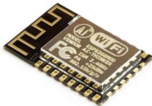
**Figura 3-19.** Microcontrolador ESP8266MOD 12E.
